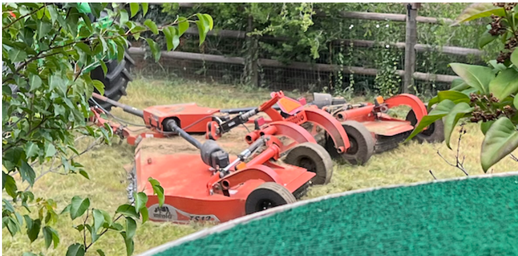
Mulching flexible blades that mow the contours of the drainage much better
